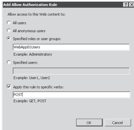
**Figure 6-26** Creating a new Allow Rule for a Web application
