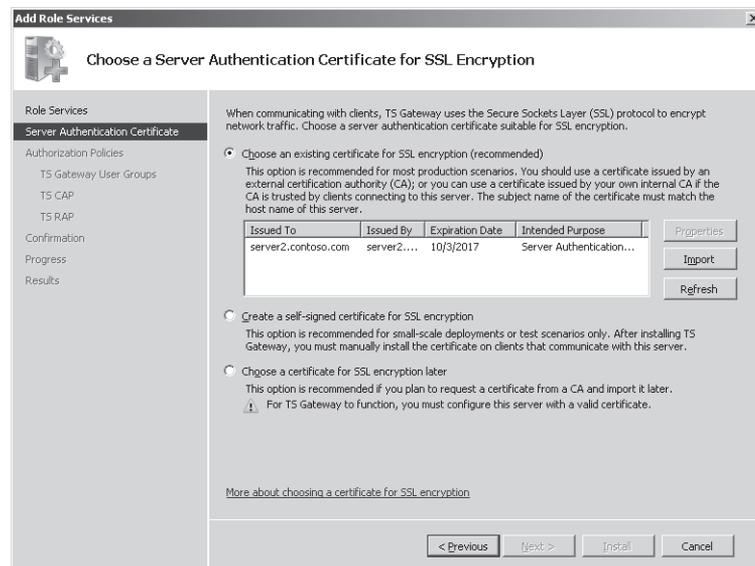
Figure 4-15 Choosing a server certificate for SSL encryption
