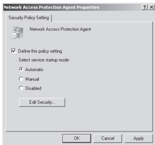
Figure 8-10 Starting the Network Access Protection Agent service automatically
